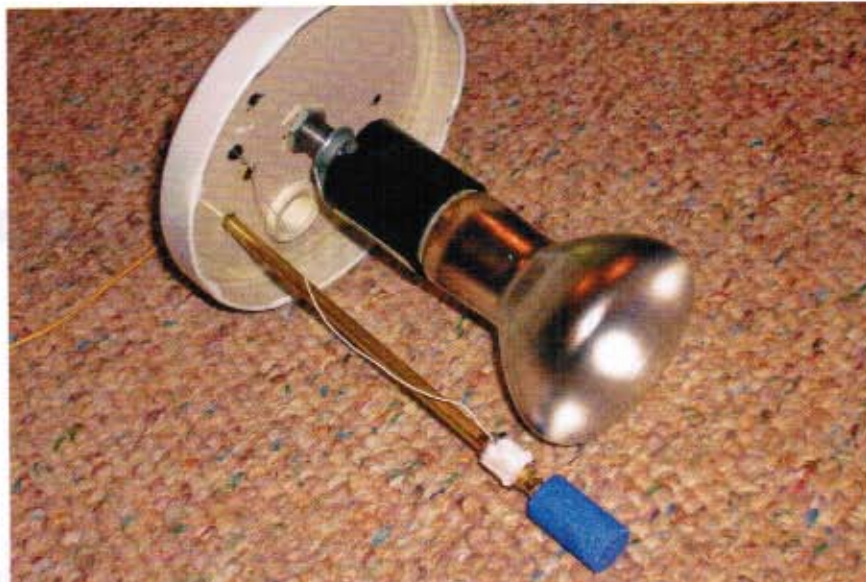
Lid with air tube/humidity sensor and lamp
