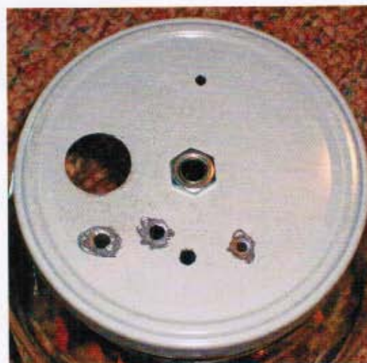
Drilled lid with paint removed at solder locations
